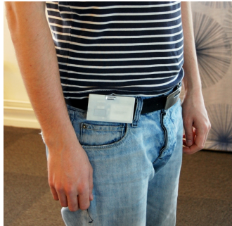
The sensors (IMU and radio) and the DSP are mounted inside an ID badge.
