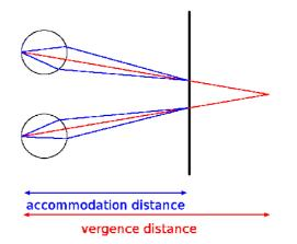
Figure 2: accommodation and vergence conflict introduced by an stereoscopic display; the virtual placement of the object is where the two red lines meet
