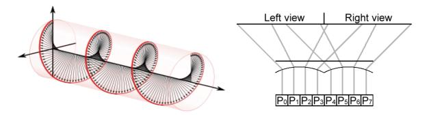
Figure 1: a) (left) polarized light wave as used in polarized-glasses-based 3D displays, taken from (wikicommons) b) (right) lenticule-based autostereoscopic display: P0..P7 donate different pixels on the display, the grey lines are the light rays emitting from these
