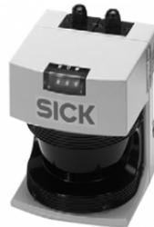
Figure 2.3: Picture of Sick LMS291
