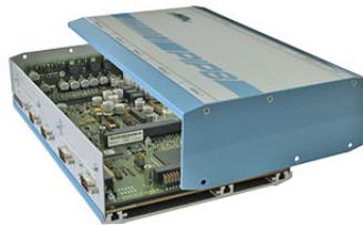
Figure 2.2: Picture of PIP8 industrial computer
