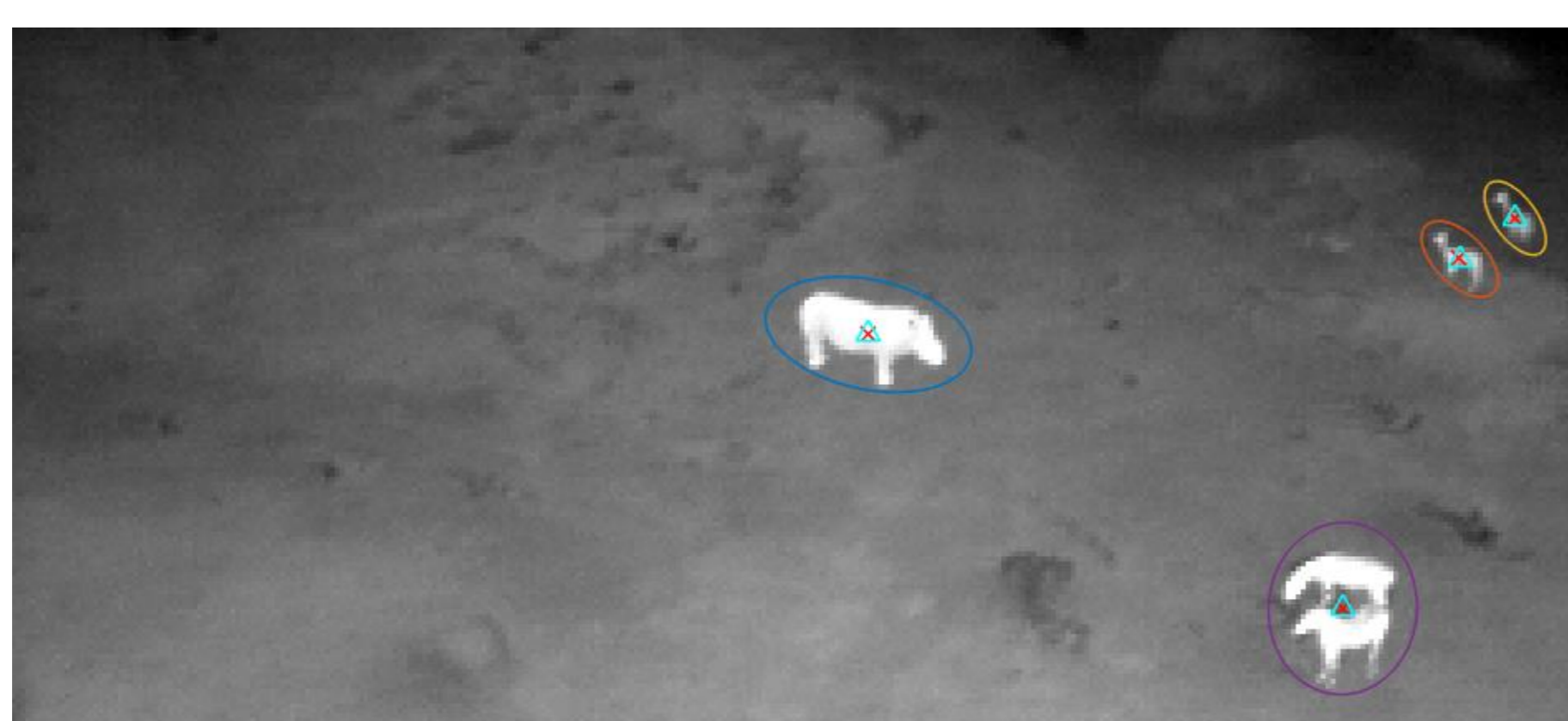
Figure 2: Extended target tracking applied to thermal camera images.
