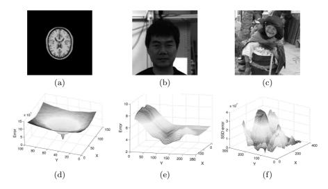
**Fig. 1.** Common test scenarios: Simple scene with constant background (a), moderate scene with background model available (b) and complex scene without background model (c). Their respective translation error surfaces are shown in (d), (e) and (f).
