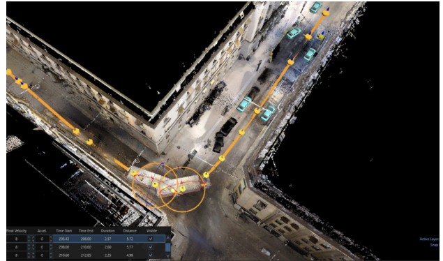
Fig. 1. 3D model of Drottninggatan, Stockholm, Sweden. The model is from registration of many terrestrial lidar scans.
