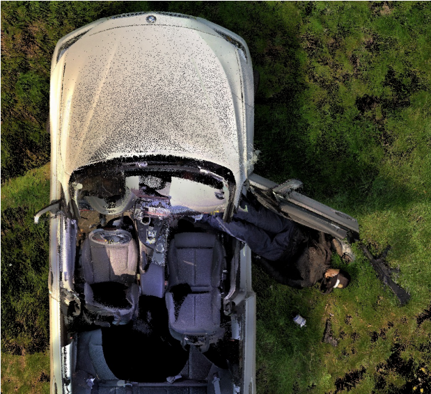
Fig. 8. 3D model from the Västervik measurement campaign created using NFC's lidar to model a scenario that illustrates a crime scene.
