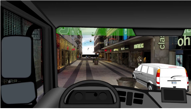
Fig. 2. 3D model of Drottninggatan as seen from the driver, Stockholm, Sweden. The model is from registration of many terrestrial lidar scans.
