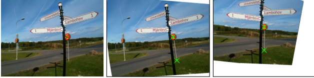
Figure 11. Image stabilisation. Left: Uncorrected RS frame. Centre: Rectified frame, with tracked points indicated. Right: Frame stabilised by centring the tracked points along a vertical line.
