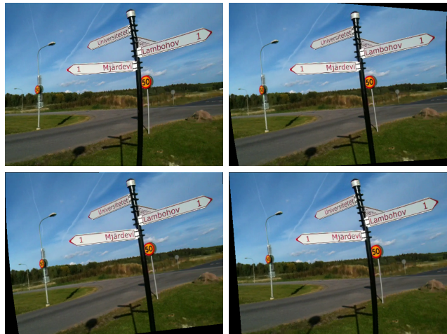
Figure 1. Example of rolling shutter imagery. Top left: Frame from an iPhone 3GS camera sequence acquired during fast motion. Top right: Rectification using our rotation method. Bottom left: Rectification using the global affine method. Bottom right: Rectification using the global shift method. Videos are available on the web and in the supplementary material.
