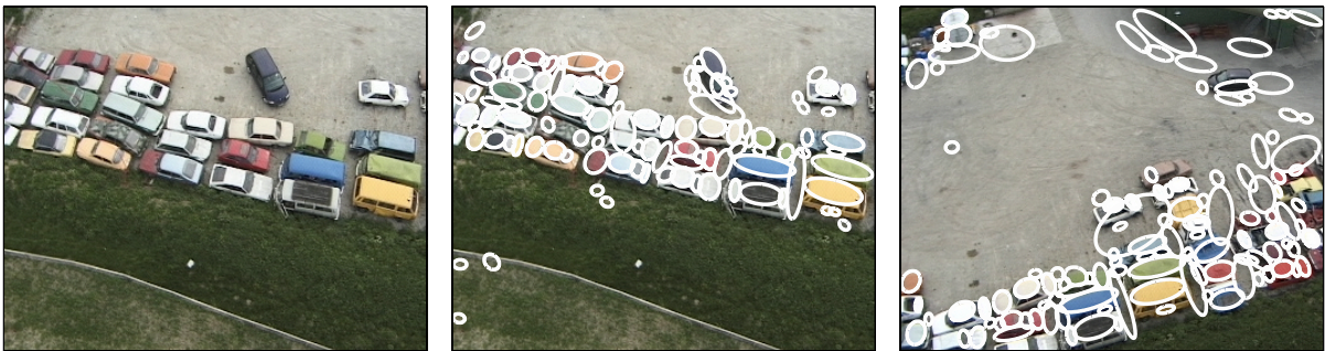
Figure 1: Blob features in an aerial image. Left to right: Input image 1, Input image 1 with detected features (107 blobs), Input image 2 with detected features (120 blobs).
