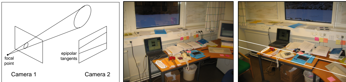
Figure 4: Epipolar constraints for ellipse. Left: cone in space generated by an ellipse in image 1 and projected into image 2. Centre and Right: The two images.
