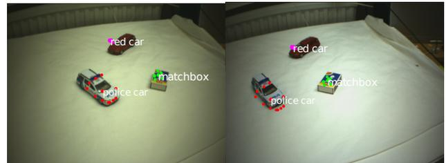
Fig. 3. Object map during system trial, objects represented by colour-coded convex hull vertices in the image plane (left view, right view)
