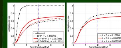
Left: Average acceptance curves over all data sets for automatically tuned CtF-BFP with  $\lambda = 0.5$ , BFP with original parameters, CtF-BFP(u) (before tuning). Errors on manually selected correspondences included as a best case.
