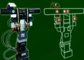
Pan-tilt stereo rig with Kinect. (A) - SLP projector, (B) - RGB camera, (C) - NIR camera, (D) - Left wide-angle camera, (E) - Right wide-angle camera, (F) - Diffusor (raised).
