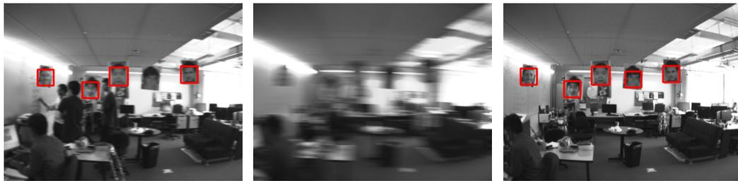
(a) Unstabilized, peak velocity  $46^\circ/\text{sec}$  (b) Unstabilized, peak velocity  $230^\circ/\text{sec}$  (c) Our stabilization method, peak velocity  $230^\circ/\text{sec}$
