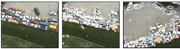
Figure 2. Blob features in an aerial image. Left to right: Input image 1, Input image 1 with detected features (107 blobs), Input image 2 with detected features (120 blobs).
