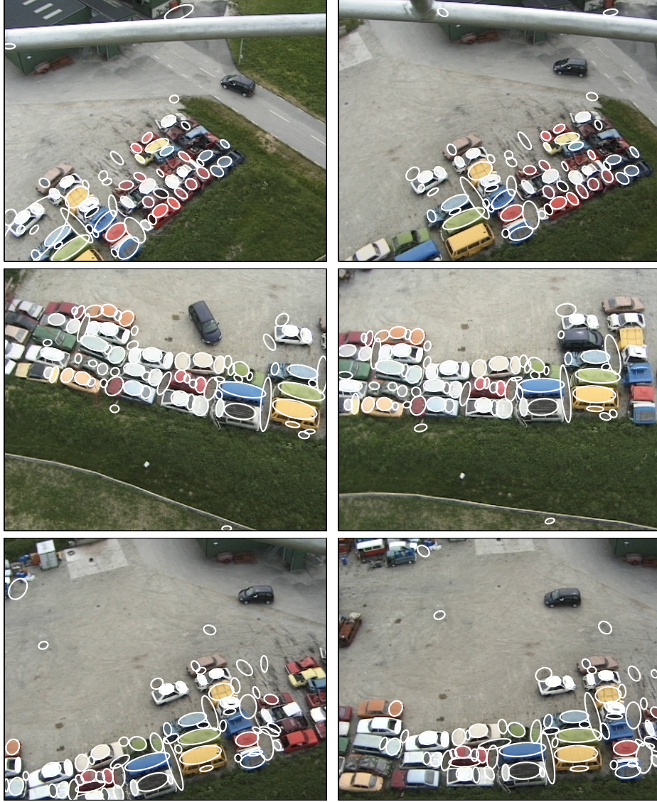
Figure 7.9: Correspondences for blobs from a video sequence. Each row shows a pair of matched images.
