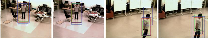
**Fig. 1.** Visualization of fusion system, the detector output is blue, tracker output green and the fused result red. The combination of both tracker and detector produces a more accurate bounding box estimate than the respective inputs, as seen in the first two frames. The last two demonstrate drift correction.
