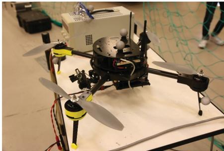
**Fig. 4.** The Linkquad UAV used to record our dataset. This configuration features a PointGrey camera and an Intel-NUC motherboard for running the vision system on board.
