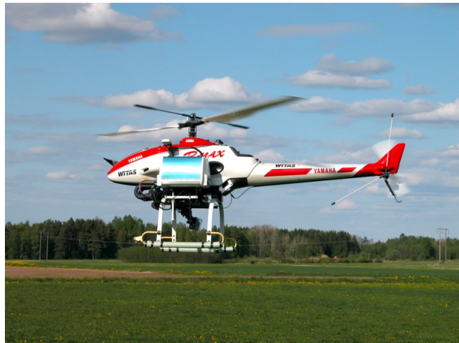
Figure 1. The Yamaha RMAX helicopter used in the experiments. The on-board system is equipped with an IMU sensor (accelerometer and gyro) and a vision sensor. The on-board GPS receiver is used for evaluation only.
