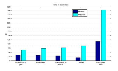
Figure 6.3: Comparison between the human driver and the autonomous system
