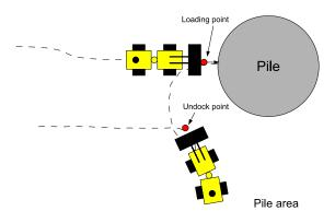
Figure 4.3: Illustration of the *fill bucket* state.
