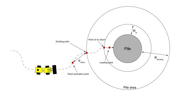
Figure 4.2: Illustration of the translation to pile state.
