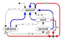
Figure B.2: Implementation of calculator using traditional state machine design.
