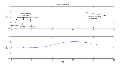
Figure 5.2: Algorithm used to create a path to a wanted position.
