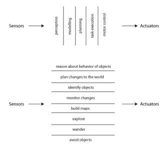
Figure 3.1: Comparison between old architecture and the subsumption architecture[2].
