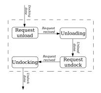
Figure 4.14: State chart of the unload bucket state
