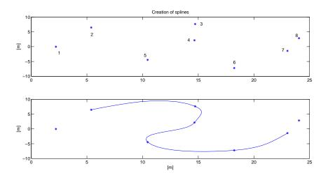
Figure 5.3: Algorithm used to smooth a sparse waypoint list.
