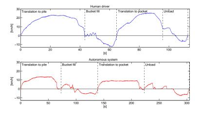
Figure 6.4: Speed comparison between human driver and the autonomous system.
