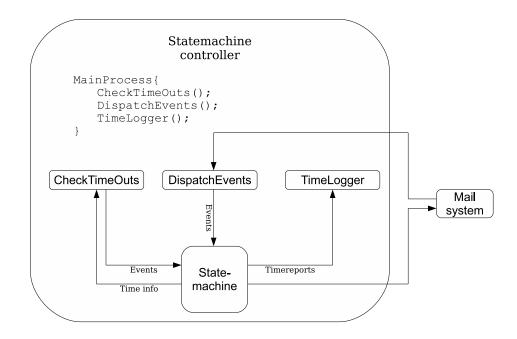
Figure 5.1: Overview of the state machine controller.
