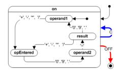
Figure B.3: Implementation of calculator using nested state machine design.
