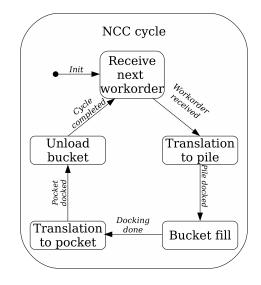
Figure 4.10: State chart of the top level in the NCC cycle
