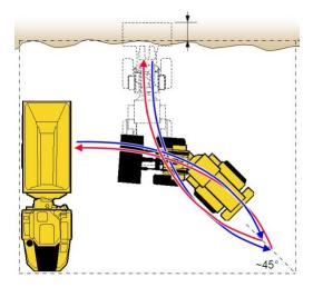
Figure 2.5: Illustration of the short loading cycle
