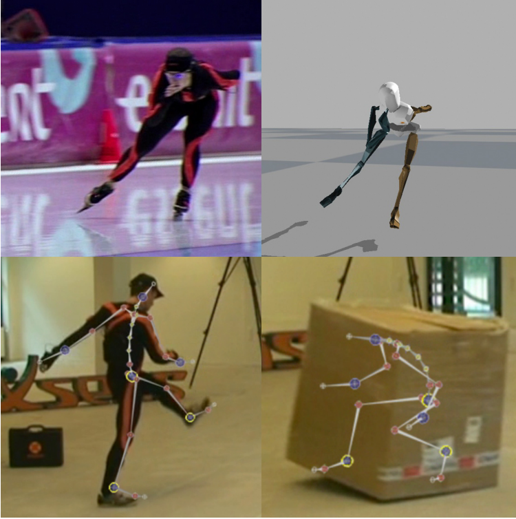
Figure 1: Examples of inertial motion capture. Upper left: olympic and world champion speed skating Ireen Wüst wearing an inertial motion capture suit with 17 inertial sensors. Upper right: graphical representation of the estimated orientation and position of the body segments. Lower left and right: experiment showing that line of sight visibility is not necessary for inertial motion capture.
