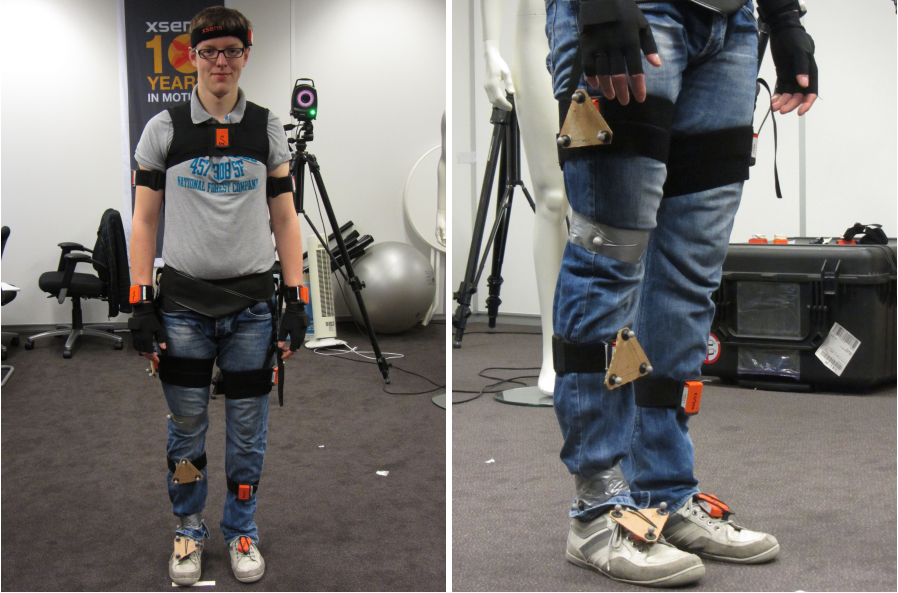
Figure 3: Experimental setup where the human body is equipped with inertial sensors on different body segments. Optical markers for the reference system have been placed on the right foot sensor, right lower and upper leg sensors and – not visible in the figure – the pelvis.
