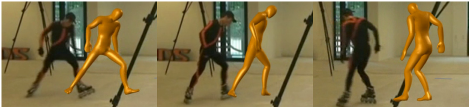
Figure 1.6: Example of inertial motion capture using 17 inertial sensors as well as 3 UWB transmitters on the head and on the feet. The estimated pose is shown in orange. By courtesy of Xsens Technologies.
