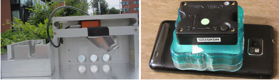
Figure 4: Left: experimental setup where a calibration experiment is performed outdoors. An Xsens MTi-100 IMU (orange box) together with a magnetic disturbance is placed in a aluminum block. Right: experimental setup using a Trivisio IMU (black box). A phone is used as a source of magnetic disturbance. To avoid saturation of the magnetometer, the phone is not attached directly to the IMU.
