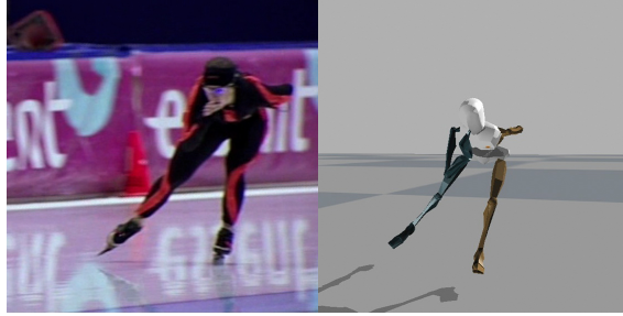
Figure 1.5: Example of inertial human body motion capture. Left: olympic and world champion speed skating Ireen Wüst wearing an inertial motion capture suit with 17 inertial sensors. Right: graphical representation of the estimated position and orientation of the body segments. By courtesy of Xsens Technologies.
