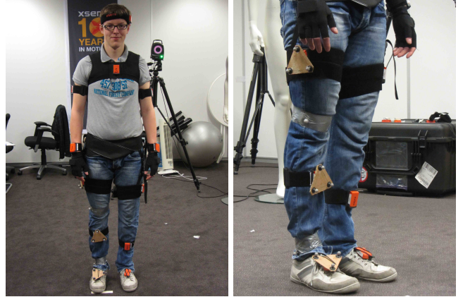
Fig. 3. Experimental setup where the human body is equipped with inertial sensors on different body segments. Optical markers for the reference system have been placed on the right foot sensor, right lower and upper leg sensors and – not visible in the figure – the pelvis.
