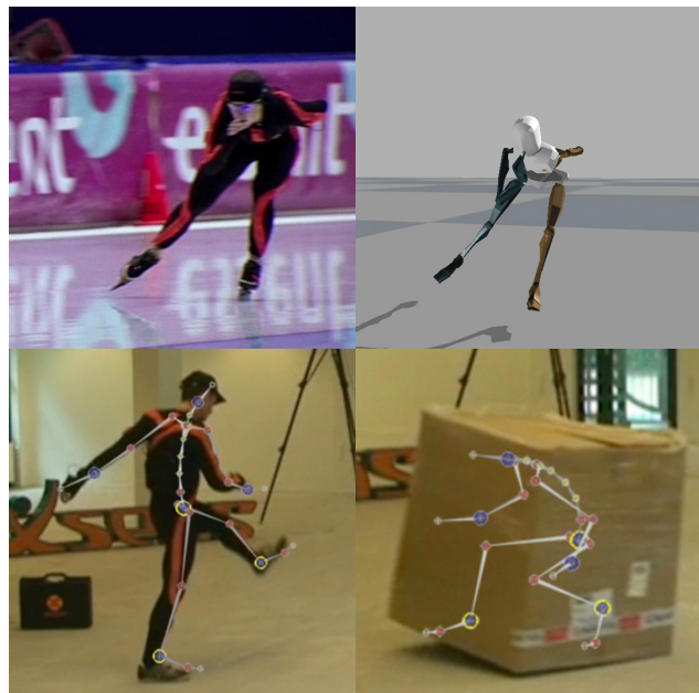
Fig. 1. Examples of inertial motion capture. Upper left: olympic and world champion speed skating Ireen Wüst wearing an inertial motion capture suit with 17 inertial sensors. Upper right: graphical representation of the estimated orientation and position of the body segments. Lower left and right: experiment showing that line of sight visibility is not necessary for inertial motion capture.
