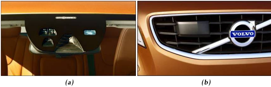
Figure 1.2: Figure (a) shows the camera and Figure (b) the front looking radar in a Volvo S60 production car. Courtesy of Volvo Car Corporation.
