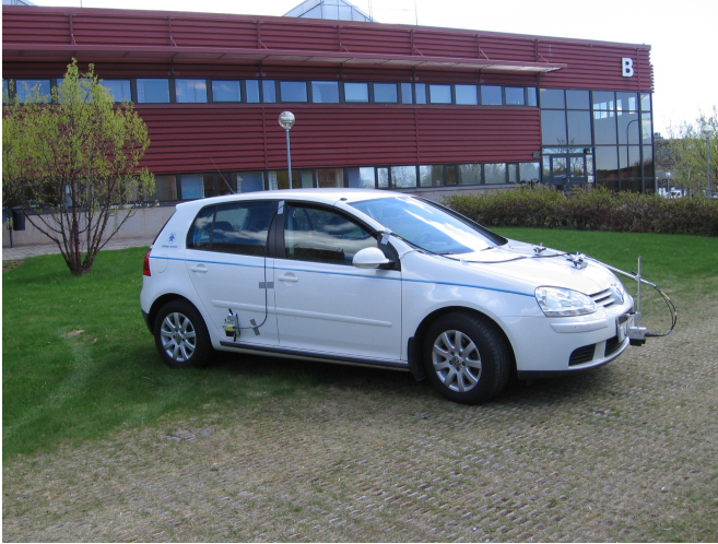
Figure 2: The test vehicle of Linköping University is logging standard CAN data. The vehicle is in addition equipped with a GPS receiver, an IMU and an optical velocity sensor.
