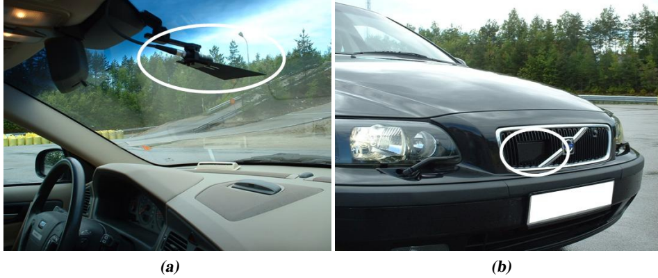
Figure 1.2: Figure (a) shows the camera in the vehicle, and Figure (b) the front looking radar. Note that this is not serial production mounting. Courtesy of Volvo Car Corporation.
