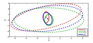
Fig. 3. Two GIW components,  $n_x = d = 2$ , merged into one component using a threshold U = 12. Shown are the kinematical state means m (dots), the corresponding covariances P (solid ellipses), and the estimated expected values of the extension state X (dashed ellipses).
