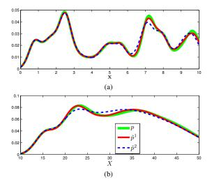
Fig. 4. Merging of 50 GIW components. (a) shows the Gaussian sum, before merging (green) as well as after merging using  $L_1$  (red) and  $L_2$  (blue). (b) shows the corresponding inverse Wishart sum. Using  $L_1$  results in 28 GIW components, using  $L_2$  results in 21 components, but also a cruder approximation.
