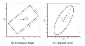
Figure 2. Relationship between target states (1) and target shape.
