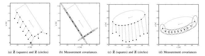
Figure 4. The rectangular and elliptical targets. (a) and (c): Example of measurements of a car and human (filled black circles), respectively, and predicted measurements located on target surface (filled black squares). The corresponding associations are shown with dashed lines. The measurement identified as being closest to the corner in the rectangular case is shown with a gray star. (b) and (d): The corresponding measurement covariances.
