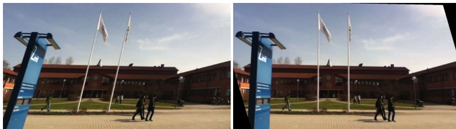
(a) Skewed image due to rolling shutter and camera turning sideways to the right. (b) Rectified image using sensors of the phone.
