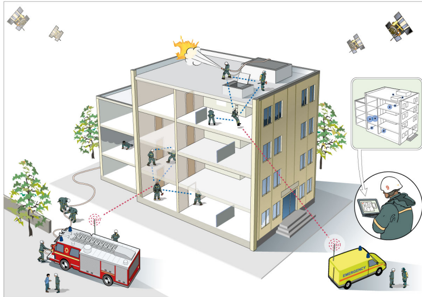
Figure 1.1: Visionary illustration of a first responder operation in an urban environment. Firefighters in the building are localized and presented for the commander in real time. Digital maps, collaborative positioning, GPS and beacons on the trucks are used to assist the positioning system. Courtesy of FOI, illustration by Martin Ek.
