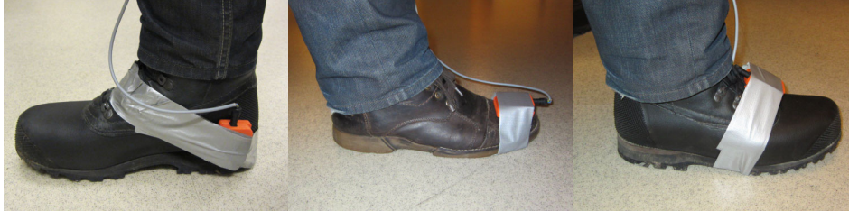
(a) Sturdy hiking boot with the sensor by the heel. (b) Softer winter boot with the sensor by the toe. (c) Sturdy boot with the sensor by the shoe laces.
