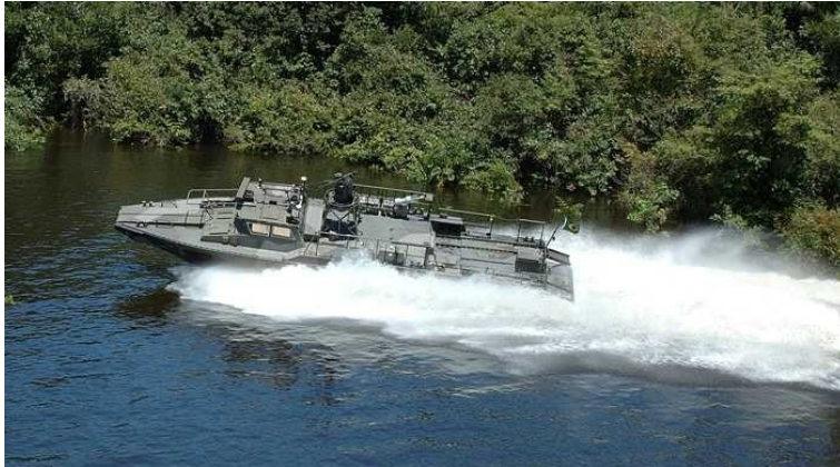
Figure 1: The high speed patrol boat type used for the data acquisition. Note the backwash created by the jet propulsion system. Courtesy of Dockstavarvet AB.
