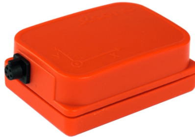
Figure 2.2: An Xsens MT motion sensor, courtesy of Xsens Technologies B.V.
