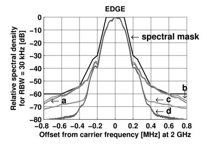
**Figure 8.4:** Measured EDGE spectrum at 2 GHz.
