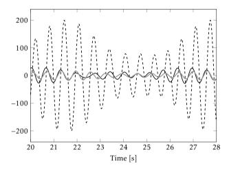
**Figure 1.2:** The input u (black solid line), and the reconstructed input  $y_u$  using an inverted estimated forward model (black dashed line) and the inverse model estimated directly (gray solid line). The estimation of the inverse (gray) cannot perfectly reconstruct the input (black solid), but is clearly better than the inverted forward model (dashed).
