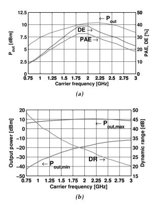
**Figure A.3:** (a) Measured output power ( $P_{out}$ ), DE and PAE over frequency. (b) Measured maximum output power,  $P_{out,max}$ , minimum output power,  $P_{out,min}$ , and dynamic range, DR, over frequency.
