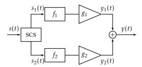
Figure 6.2: A schematic picture of the amplifier branches setup. Note that the functions  $f_k$ , k = 1, 2, are not functions of the input to the block only but are used to show the general functionality of the PA with the separation of the two branches.
