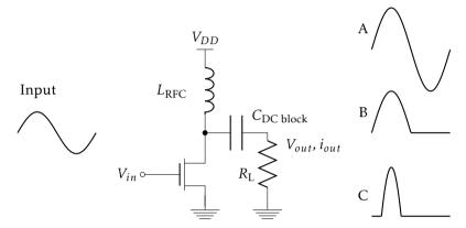
**Figure 5.10:** Generic Class A/B/C power amplifier. The biasing of the transistor determines the conduction angle of the PA, as illustrated in the amplification of a sinewave input (left). The conduction angles are (from top to bottom) 360° for the Class A, 180° for the Class B and 90° for the Class C here.
