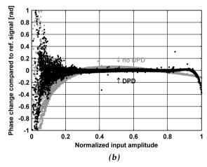
**Figure 8.7:** (a) Measured AM-AM characteristics (output amplitude vs. input amplitude) with DPD (black) and without DPD (gray) for WCDMA signal. (b) Measured AM-PM characteristics (phase change vs. input amplitude) with DPD (black) and without DPD (gray) for WCDMA signal.
