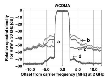
Figure 8.5: Measured WCDMA spectrum at 2 GHz.
