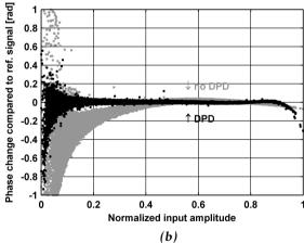
**Figure 8.9:** (a) Measured AM-AM characteristics (output amplitude vs. input amplitude) with DPD (black) and without DPD (gray) for LTE signal. (b) Measured AM-PM characteristics (phase change vs. input amplitude) with DPD (black) and without DPD (gray) for LTE signal.
