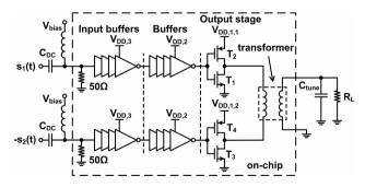
**Figure A.2:** Implemented outphasing amplifier with inverters in the output stage.
