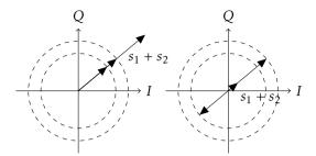
**Figure 5.15:** The outphasing concept when the gain factors  $g_1$  and  $g_2$  are not identical. In the left figure, the outphasing signals are parallel and the resulting output is the maximal one. In the right figure, the nonidentical gain factors cannot cancel each other, and some remains are left. The dynamic range (the ratio between the maximal and minimal amplitudes, see (5.13)) of the power amplifier will determine the limit of small amplitude clipping.
