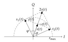
Figure 5.12: Outphasing concept and signal decomposition.
