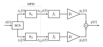
**Figure 7.1:** A schematic picture of the amplifiers with predistorters. Note that the functions  $f_k$  and  $h_k$ , k = 1, 2, are not functions of the input to the block only, but are used to show the general functionality of the PA and the DPD with the separation of the two branches.
