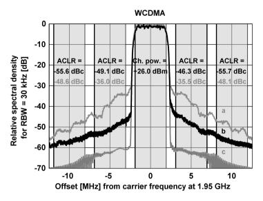
Figure 8.6: Measured WCDMA spectrum at 1.95 GHz.
