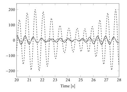
**Figure 4.4:** The input u (black solid line), and the reconstructed input  $y_u$  using the inverted forward model (black dashed line) and the inverse model estimate using METHOD C (gray solid line). The estimation of the inverse cannot perfectly reconstruct the input, but is clearly better than the inverted forward model.
