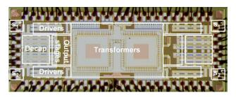
**Figure A.4:** Photo of the chip with size 2.5x1.0mm<sup>2</sup>. The photo has the same orientation as the simplified PA schematic in Figure A.5.
