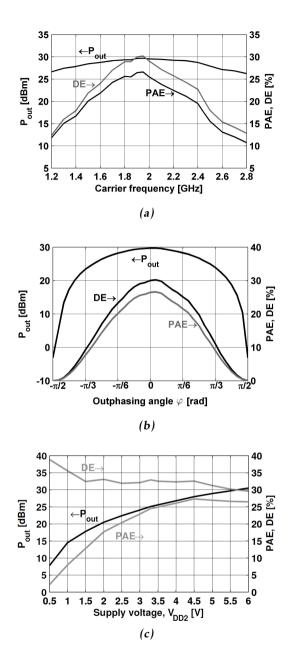
**Figure A.7:** Measured  $P_{out}$ , DE and PAE for  $V_{DD1} = 1.3 \text{ V}$  and  $V_{DD2} = 5.5 \text{ V}$  [Fritzin et al., 2011c]:
