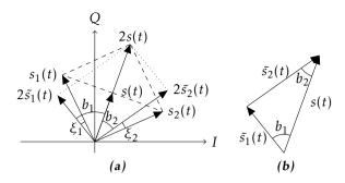
**Figure 6.1:** (a) Decomposition of the input signal s(t) into  $s_1(t)$  and  $s_2(t)$  when  $g_1 = g_2 = g_0 = 0.5$  and into  $\tilde{s}_1(t)$  and  $\tilde{s}_2(t)$  when decomposed as in (6.3) with nonidentical gain factors  $g_1$  and  $g_2$ . (b) Trigonometric view of the decomposition of s(t) using nonidentical gain factors. Note that  $|\tilde{s}_k| = g_k, k = 1, 2$ .
