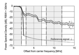
**Figure 5.14:** The bandwidth of the quadrature signal e(t), and thus the outphasing signals  $s_1(t) = s(t) + e(t)$  and  $s_2(t) = s(t) - e(t)$ , is much larger than that of the original signal s(t). Any remainders of the quadrature signal caused by PA imperfections will thus lead to degraded ACLR and reduced margins to the spectral mask. From Fritzin [2011].
