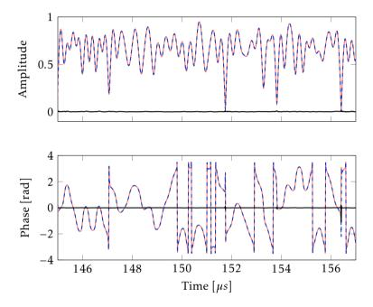
**Figure 6.5:** Model validation of the model produced using the convex method in (6.18)-(6.19) and the dynamic range has been used to determine the gain factors as in (6.17) and (6.15). The upper plot shows the amplitude of the measured signal (solid pink), the model output (dashed blue) and the error (black line). The lower plot shows the phase.
