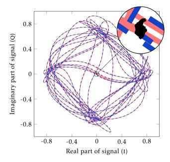
**Figure 6.8:** IQ plot (imaginary part, Q, vs real part, I) of the measured signal (solid pink) and the model output (dashed blue) and the error  $y - \hat{y}$  (black). The model was estimated by the LS method using DR to estimate  $g_1$  and  $g_2$ . The zoom-in in the upper right corner is a ten times amplification of the error signal.
