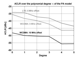
**Figure 8.10:** Measured ACLR depending on the polynomial degree n of the PA model. Degree n = 0 represents the performance without predistortion. The nonlinear modeling and distortion clearly improves the performance by reducing the ACLR.
