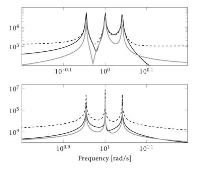
**Figure 4.5:** Periodogram of the input u (black solid line), and the reconstructed input  $y_u$  using the inverted forward model (black dashed line) and the inverse model estimate using METHOD C (gray solid line) around  $\omega = 1$  rad/s (top) and  $\omega = 10$  rad/s (bottom). It is clear also in the frequency domain that the forward model better captures the behavior around  $\omega = 1$  rad/s than the inverse estimation, but the reverse is true around  $\omega = 10$  rad/s.
