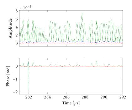
**Figure 7.4:** The upper plot shows the amplitude error,  $|s - \hat{y}_p|$ , and the lower plot shows the phase error,  $\arg(s) - \arg(\hat{y}_p)$ , for the two DPD methods. The analytical method is in pink and the LS in blue. As a comparison, the errors for the original, unpredistorted signal y(t) are also plotted in green.
