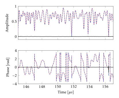
**Figure 6.4:** Model validation of the model produced using the original, nonconvex, optimization in (6.12)-(6.14). The upper plot shows the amplitude of the measured signal (solid pink), the model output (dashed blue) and the error (black). The lower plot shows the phase.
