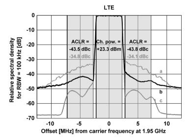
Figure 8.8: Measured LTE spectrum at 1.95 GHz.
