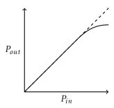
**Figure 5.8:** Gain compression due to saturation in an amplifier transistor. The dashed line represents the ideal operation of the amplifier, while the solid line is the true output of the PA and a consequence of gain compression.
