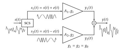
**Figure 5.13:** Illustration of ideal power combining (the plus sign) of the two constant-envelope signals. The signals are amplified separately by two nonlinear amplifiers,  $A_1$  and  $A_2$ , and recombined to an amplified replica of the input s(t).
