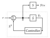
**Figure 3.5:** A block diagram of Hirschorn's method, where the system S is replaced by a model  $\hat{S}$  in the exact linearization feedback loop. The input signal calculated in this way is then also applied to the real system S. The simulation system and feedback loop that leads to an overall linear behavior between r and  $y_s$  is denoted  $S^{\dagger}$ . The input to  $S^{\dagger}$  is the reference r and the output is the control signal u.
