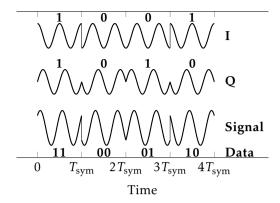
**Figure 5.4:** The modulated signals in the IQ modulation, where the two carrier waves are sinusoidal with a 90° phase shift. The odd-numbered bits encode the in-phase (I) component and the even-numbered bits encode the quadrature (Q) component. The total signal is shown at the bottom, together with the mapping. The digital data transmitted by this signal is  $1\ 1\ 0\ 0\ 0\ 1\ 1\ 0\ .\ T_{\text{sym}}$  is the symbol duration.
