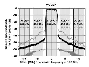
**Figure 5.6:** Spectrum at 1.95 GHz for (a) measured output without DPD, (b) measured output with predistortion (linearization) and (c) the input signal for a WCDMA signal. The measured ACLR are printed in gray for the original output signal (without predistortion) and in black for the predistorted output. The gray shadows represent the passband in which the integration takes place.
