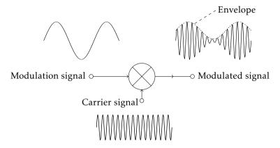
**Figure 5.2:** Amplitude modulation. The information in the modulation signal is upconverted in the mixer to the carrier frequency (frequency of the carrier signal) and the shape (envelope) of the modulated signal contains the original information in the modulation signal.
