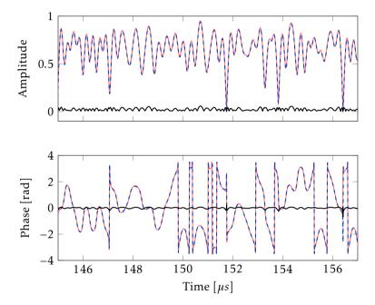
**Figure 6.3:** Model validation of the model produced using the first structure (6.8), with gain factors  $g_1$  and  $g_2$  and a phase shift  $\delta$  only. The upper plot shows the amplitude of the measured signal (solid pink), the model output (dashed blue) and the error (black). The lower plot shows the phase.
