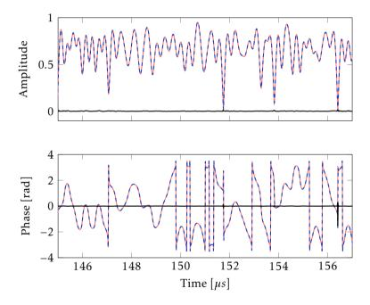
**Figure 6.6:** Model validation of the model produced using the convex method in (6.18)-(6.19) and  $g_1$  has been gridded in  $[g_{min}, g_{max}] = [0.4, 0.6]$  with precision  $p_M = 0.005$ . The upper plot shows the amplitude of the measured signal (solid pink), the model output (dashed blue) and the error (black line). The lower plot shows the phase.
