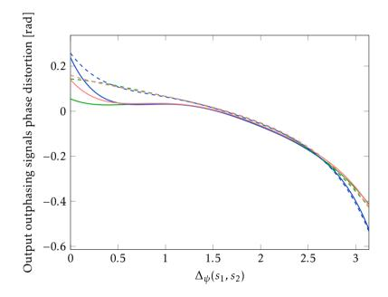
**Figure 6.10:** Simulated outphasing output phase distortion of the models from the nonconvex method (green) and the LS methods using DR (blue) and gridding (pink). The lines describe the modeled phase in each branch as a function of the input signal amplitudes. Branch one is plotted in solid lines and branch two in dashed lines.
