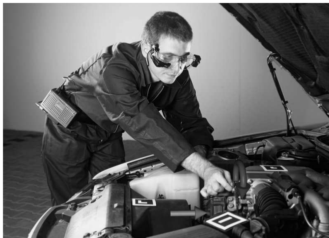
Figure 1.2: Augmented reality is used to give instructions for the assembling of a car. Courtesy of Fraunhofer IGD.
