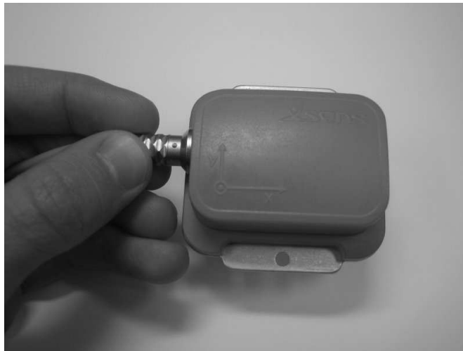
Figure 5.1: The IMU MTi from Xsens Technologies which is used for the experiments in this thesis.
