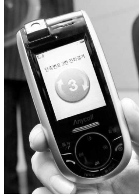
Figure 1.3: Cell phone from Samsung with built in accelerometers and magnetometers.
