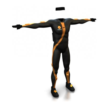
17 sensor units are mounted onto the body of the person.
