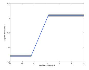
Fig. 4. Estimated (grey) and true (blue) memoryless nonlinearities for the example studied in Section 5.
