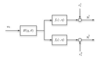
Fig. 2. Block diagram of blind Wiener model with two outputs.
