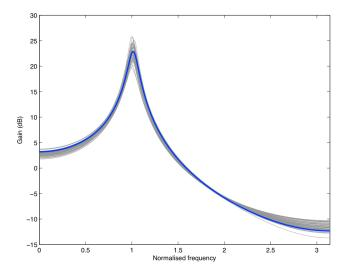
Fig. 3. Bode plot of estimated (grey) and true (blue) systems for the example studied in Section 5.
