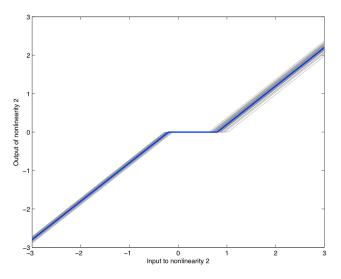
Fig. 5. Estimated (grey) and true (blue) memoryless nonlinearities for the example studied in Section 5.
