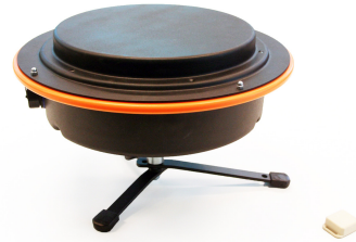
Fig. 3. Hardware used in an UWB setup. More specifically, an UWB receiver and a small, battery-powered UWB transmitter.
