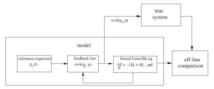
Fig. 10. Block diagram for the "model-based feedback" control design.
