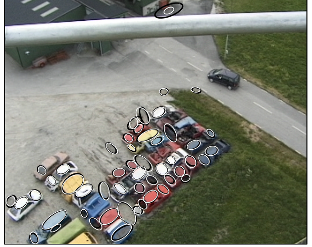
Figure 4: Blob shapes projected through the homography. Original blob shapes are black ellipses, projected shapes are white.
