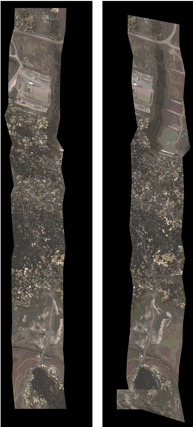
Fig. 7. Result for aligning the two strips from the first flight path, with N = 21 , and regularisation parameter \alpha = 60\,000 .
