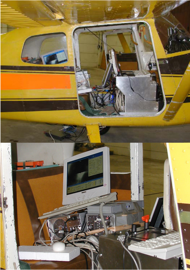
Fig. 1. The sensor installation in the aircraft. Top: The sensors are installed in the metal box beside the pilot. Bottom: Computer and storage equipment in the back seat.
