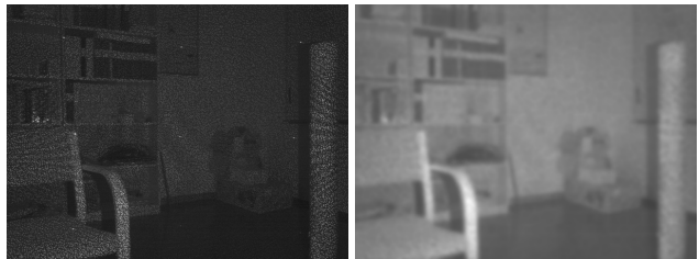
Figure 2. Removal of structured-light pattern in NIR image. Left: input image (gamma corrected) Right: result of pattern removal.
