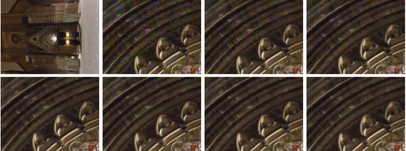
Figure 5. Scene captured using a physical tripod. Left to right, top to bottom: denoised image using 64 frames, zoomed in detail using 1, 2, 4, 8, 16, 32 and 64 frames respectively. (Best viewed electronically)
