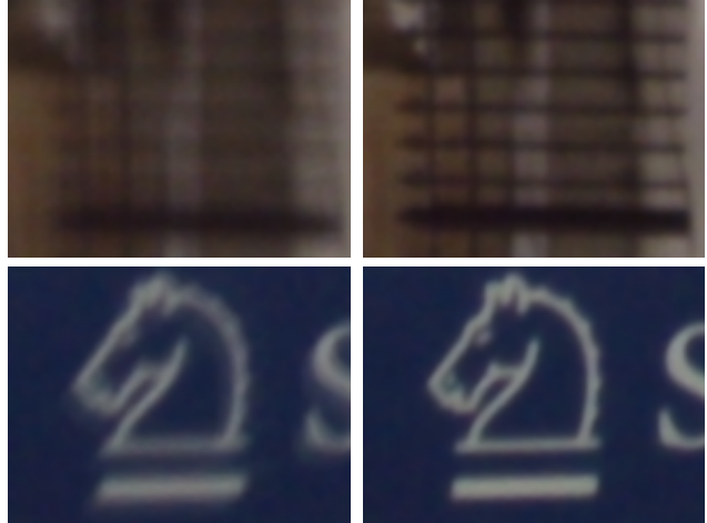
Figure 3. Zoomed in examples between global frame alignment (left) and our rolling shutter aware method (right). For full frames, see Figure 7, top left, and Figure 6, bottom left.
