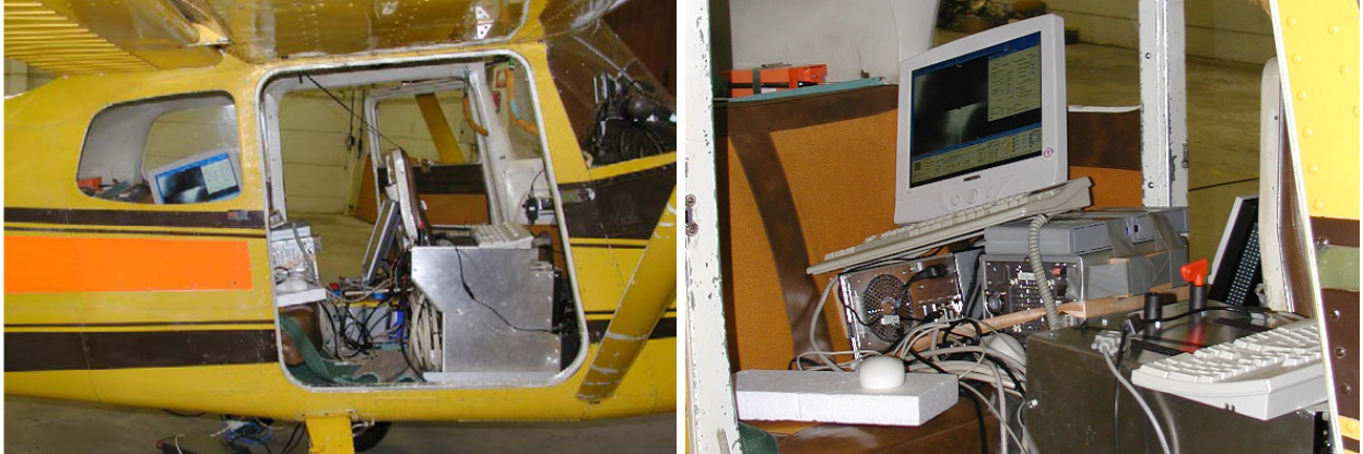
Figure 1. The sensor installation in the aircraft. Left: The sensors are installed in the metal box beside the pilot. Right: Computer and storage equipment in the back seat.
