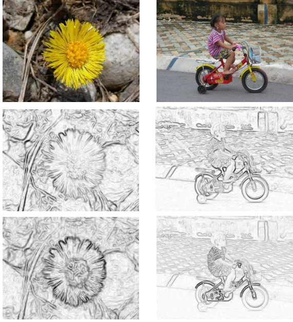
Figure 3: Comparison for edge detection. Top row: Original images. Middle row: RGB color edges. Bottom row: color-boosted edges. RGB edges are more biased by luminance.
