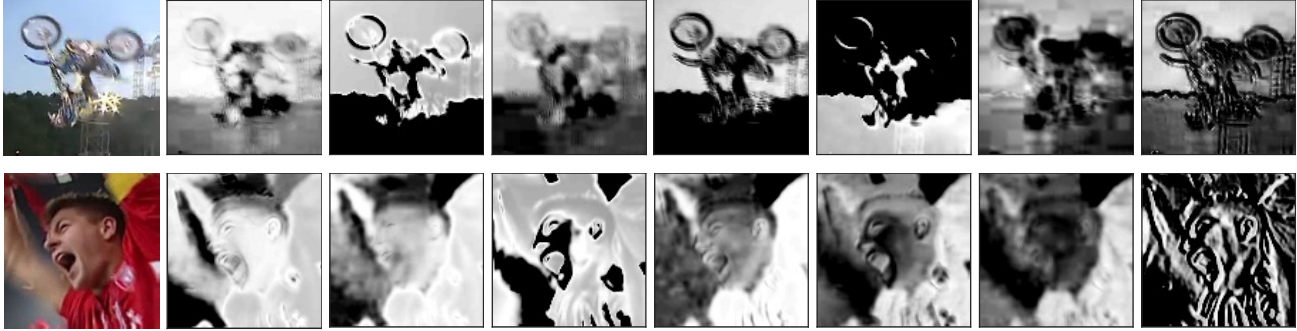
Figure 4. Visualization of the employed first-layer convolutional features with the highest energy. Activations are shown for two sample patches (left), taken from the motorBike (top row) and soccer (bottom row) sequence respectively. The convolutional features capture different colors and edges over image regions.
