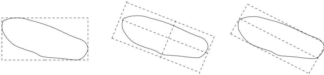
**Figure 3.7** The three different types of bounding boxes. From left to right: axis aligned, PCA and minimum volume
