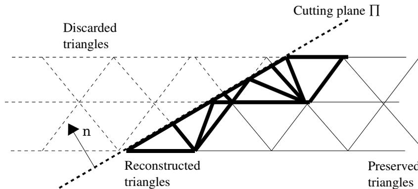
**Figure 3.8 Cut and reconstruct process. Reconstructed triangles (bold) together with the triangles under the plane form the new object's surface.**
