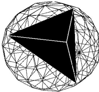
**Figure 6.22** A bounding sphere that encloses a tetrahedron as an attempt to introduce a richer variety of normal orientations.
