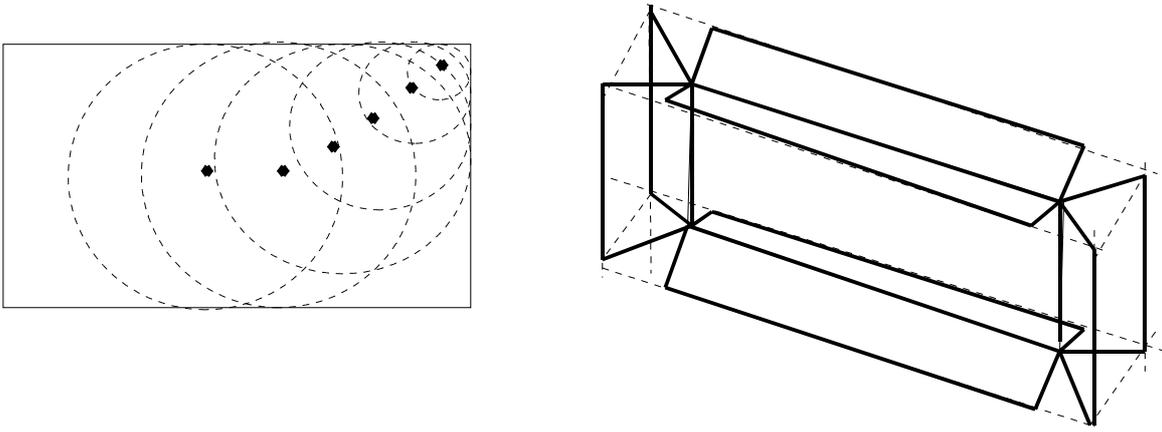
**Figure 2.1 Left: Maximal circles interior to the rectangle with their centres. The centres are points on the medial axis. Right: 3d medial surface of a box**
