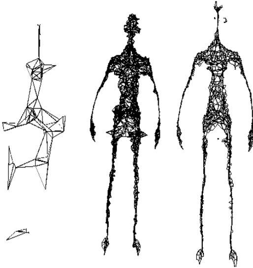
Figure 6.13 The medial axis of a 292 triangle model produced by *Powercrust* (left), the medial axis of a 500 triangle model by *Powercrust*(middle) and the medial axis from the same model by *Tight-Cocone* (right).
