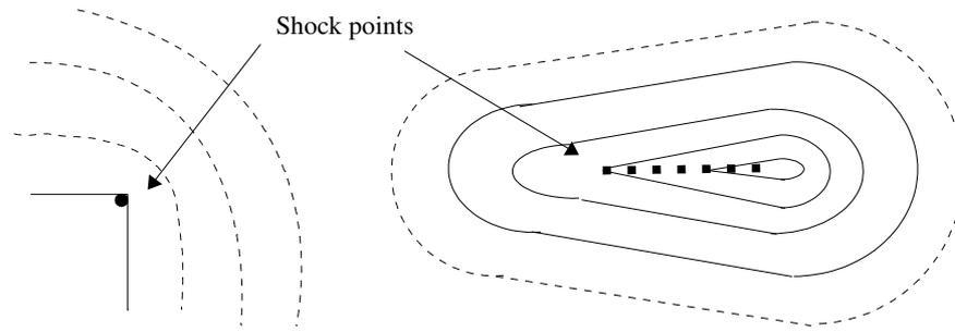
**Figure 3.6 Shock points (thick dots) generated from the erosion of the curve**
