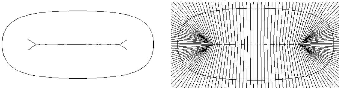
**Figure 2.3** On the left a convex curve and its medial axis, and on the right the Voronoi diagram of the curve, together with its approximated medial axis.
