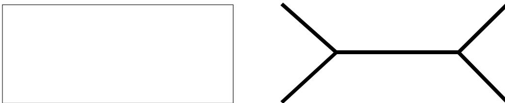
**Figure 1.1** A rectangle (left) and its medial axis (right)
