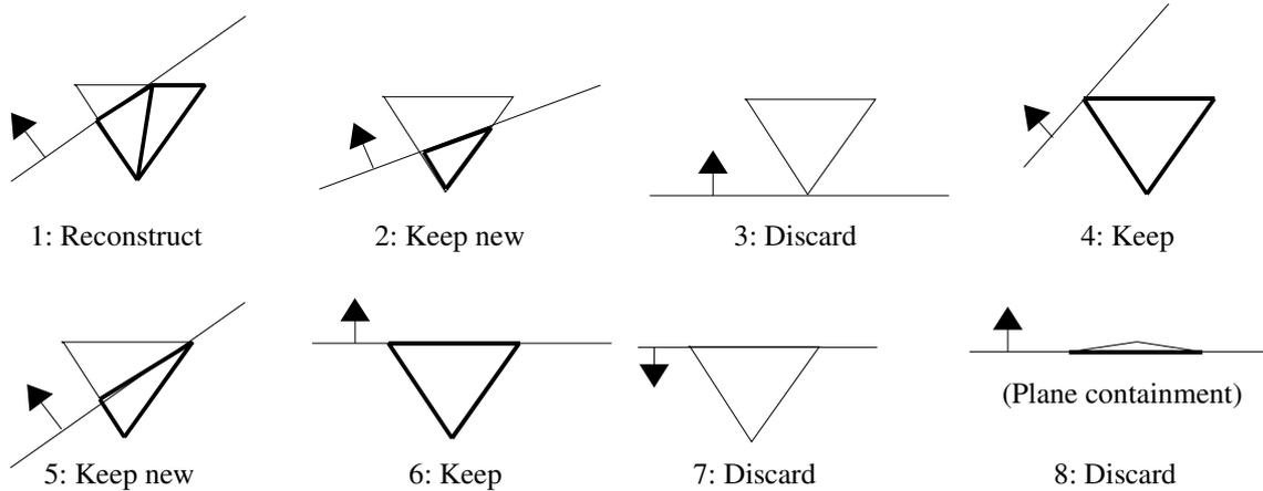
**Figure 3.9** The eight possible ways a triangle can intersect with a plane and how it can be reconstructed
