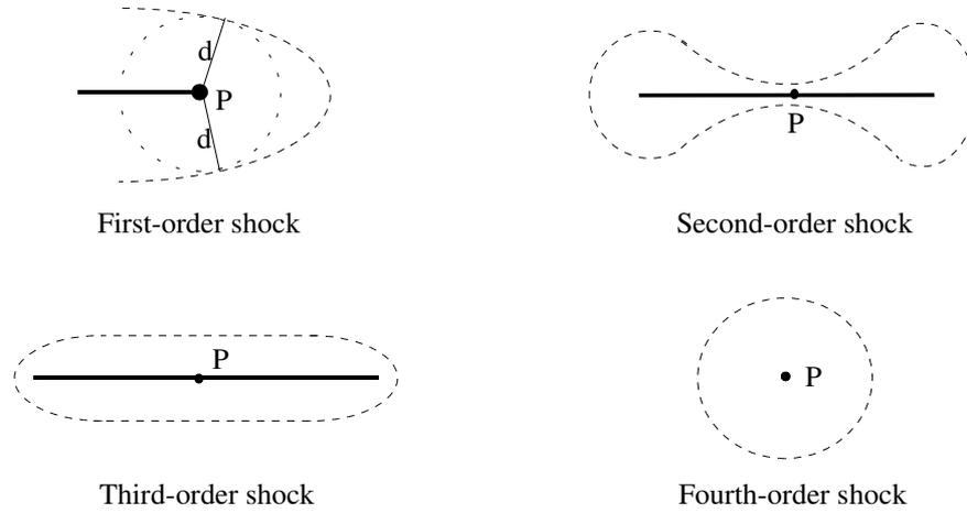
**Figure 3.12 The four types of shocks created during the deformation process**
