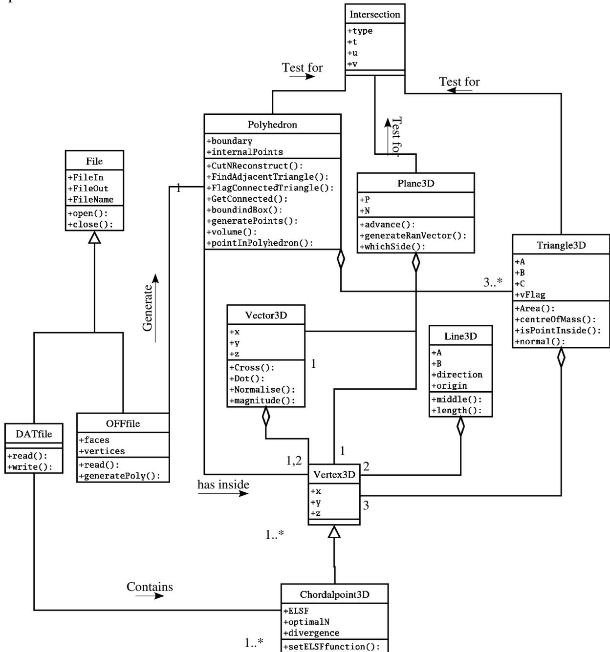
Figure 4.1 Class diagram of the skeletonisation system
