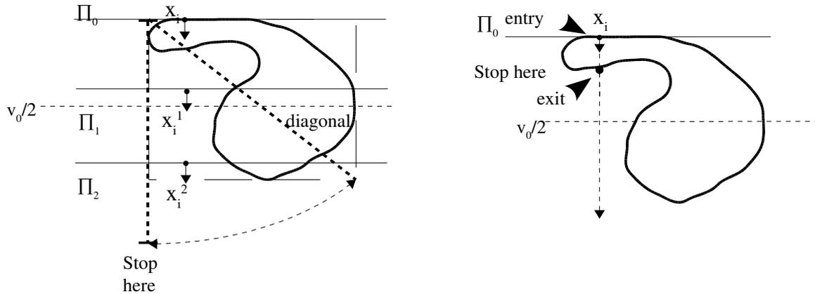
**Figure 3.11** Some solutions to the forever advancing plane problem. Using the diagonal distance (left) and ray-casting to detect entry and exit points (right). It is obvious that from the example sketched, the ray-casting method is in principle far superior to the diagonal distance.
