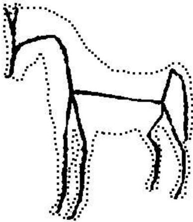
**Figure 2.4** Reeb skeleton (bold) of real 3d data (only the boundary of the object is shown here for simplicity)
