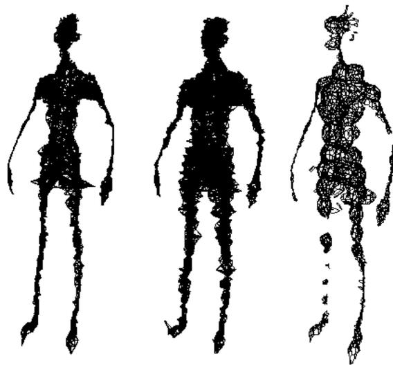
**Figure 1.4 Skeleton from a body scan (left) and skeletons after addition of surface and volumetric noise the the scan (centre and right respectively).**
