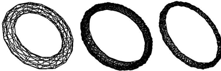
**Figure 3.5** Original torus (left) with volume  $v_0$ , affine erosion with a threshold  $v_0/10$  (middle) and with a threshold of  $v_0/7$  (right).
