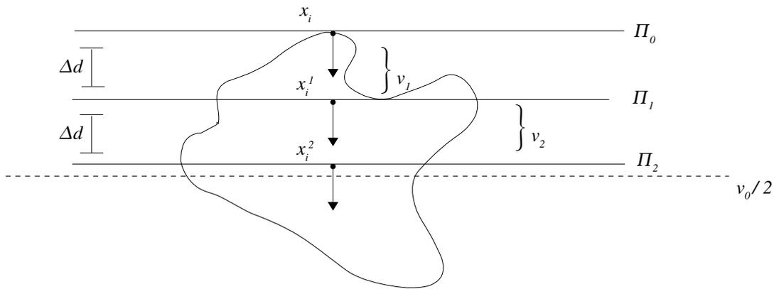
**Figure 3.4** We advance the cutting plane and calculate the chordal volumes until we reach  $v_0/2$
