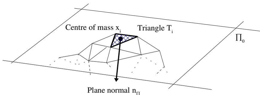
**Figure 3.2 Starting point of the algorithm, creating the cutting plane**
