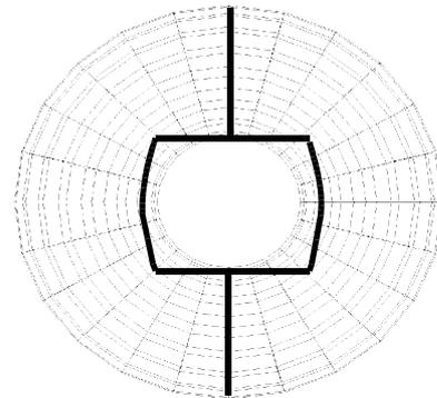
**Figure 2.5** Reeb graph of a torus (bold lines). The graph will correspond to the topology of the object.
