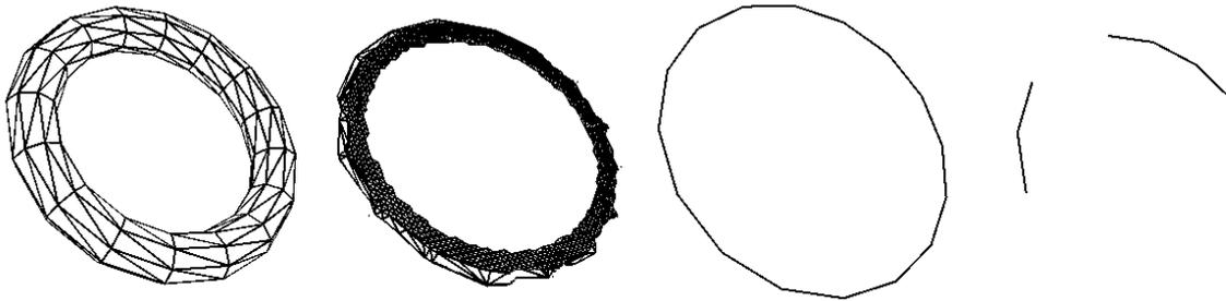
**Figure 6.1** (Left) A triangulated torus, (second from left) its affine skeleton, (second from right) medial axis approximated by *Tight-Cocone* and (right) medial axis approximated by *PowerCrust*.
