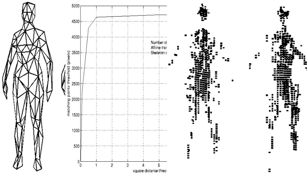
**Figure 6.19** The original skeleton of the original body (left) and its affine transformation (right). **Figure 6.20** The affine transformed skeleton of the original body (left) and the affine skeleton of the body deformed by the same affine transformation (right). **Figure 6.21** The similarity graph of the two skeletons.
