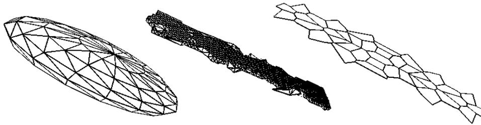
**Figure 6.4** On the left a triangulated ellipsoid and its affine skeleton (middle). On the right we see an approximation of its medial axis by the *Tight-Cocone* software.
