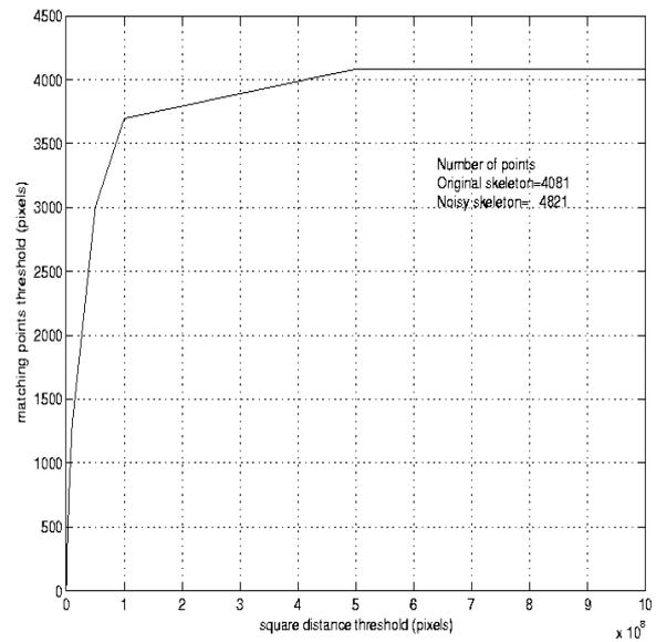
**Figure 6.18** The similarity graph plot for the original and noisy skeletons, as computed by *Powercrust*.
