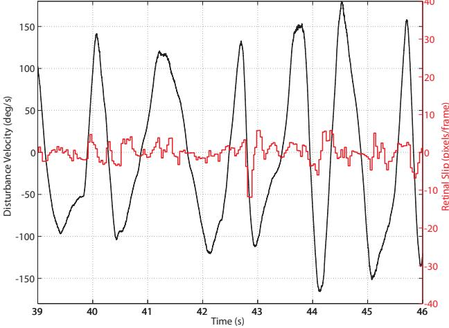
Figure 9: System performance to a user-driven disturbance. The disturbance velocity is obtained directly from the angular rate measurement of the IMU.
