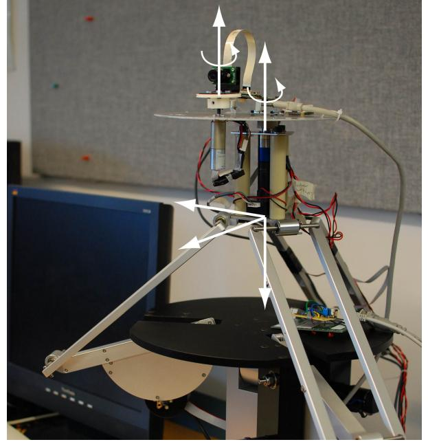
Figure 3: The head platform mounted on the robotic test platform with the axes of motion indicated. The camera head is actuated by a DC motor allowing a rotation about an axis perpendicular to the ground. The test platform rotational axis (at the neck joint) is parallel to the camera’s and is colinear to one of its translational axis.
