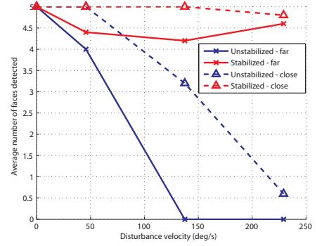
Figure 11: Relationship between disturbance velocity and face detection performance when all 5 printed faces are within field of view. Each data point corresponds to an average of over 5 samples, ignoring false positives.
