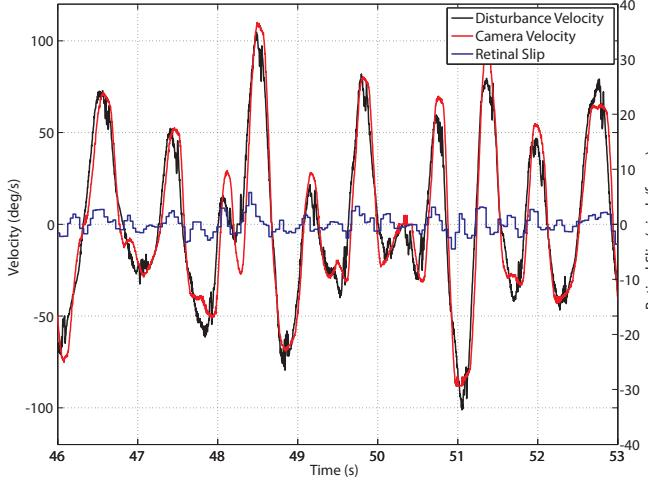
Figure 6: System performance to a bandpass noise disturbance. The sign of the camera velocity has been changed for easier visualization.
