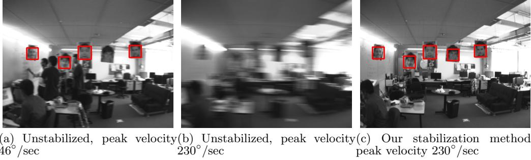
Figure 10: Image frames with faces, captured by the camera (60 fps) with and without stabilization. Detected faces are marked with a red box. Our system performs well even at 230°/sec.
