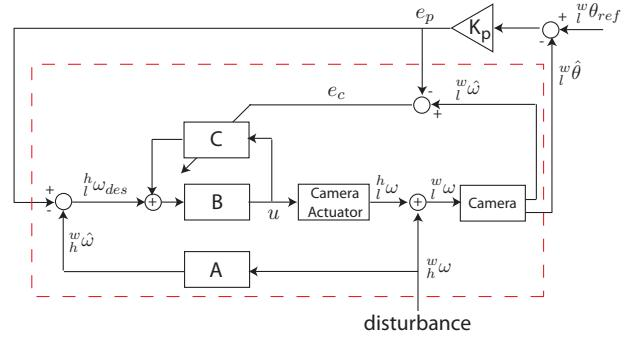
Figure 4: Our gaze stabilization architecture consisting of the velocity tracking inner loop (inside the dashed box) and a position tracking outer loop. The angular rate inertial sensor (A) provides an estimate of the rotational velocity of the head platform. In our Cerebellum-like recurrent design, the desired camera velocity is augmented with the output of the cerebellum (C) and used by the brainstem (B) to generate the plant control signal ( $u$ ).
