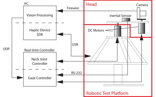
Figure 2: Overview of the hardware setup used to test the gaze control algorithm. The gaze controller uses only the visual, inertial, and camera position information to compensate the camera motion generated by the test platform.
