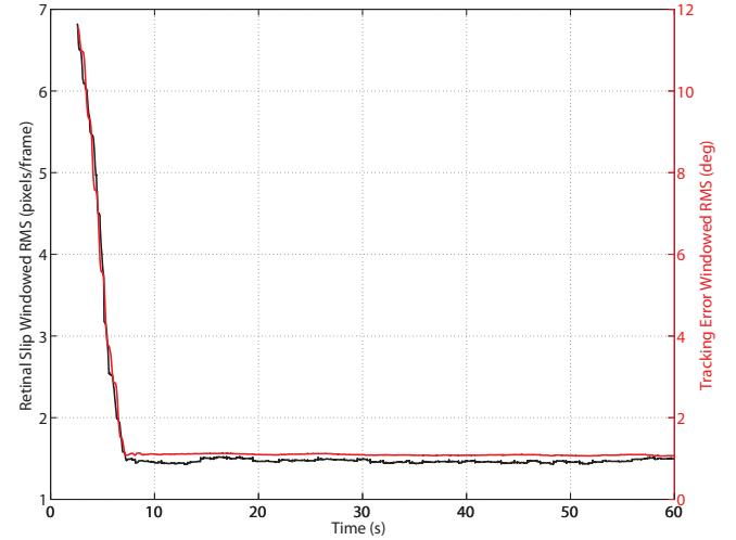
Figure 7: With the brainstem gain set to 50% of the correct value. Position and velocity tracking RMS error (with 5 seconds window) to a sinusoidal disturbance signal with a maximum velocity of  $230^\circ/\text{sec}$
