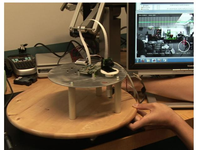
Figure 8: The wheeled-platform used to subject our gaze-stabilization system with user-driven disturbance.
