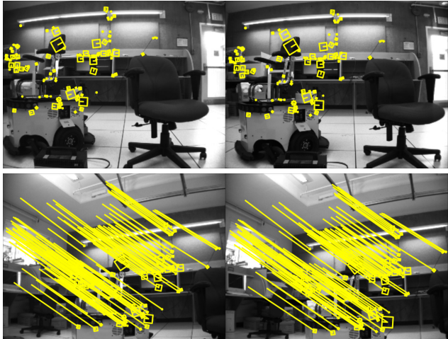
Figure 2. Feature matching across a saccade. Top: Stereo pair before saccade, with matched SIFT features painted in. Bottom: Stereo pair after saccade, with 114 estimated feature motion vectors painted in. The saccade shown has a pan change of 20^\circ and tilt change of 14^\circ . Each image has a 640 \times 480 resolution.
