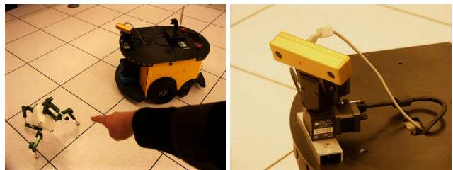
Figure 1. Using gaze instead of pointing to indicate an object of interest. Left: Robot and person indicating a common object of interest. Right: Close-up of the pan-tilt stereo head.
