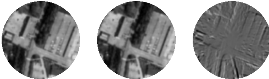
Figure 5.7: Images after alignment, and the difference image.
