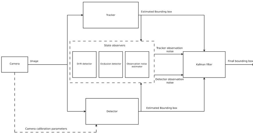
**Fig. 2.** An overview of the tracking system, the details of the tracker are described in Sect. 3.1, the detector in Sect. 3.2 and the observer components in Sect. 3.4
