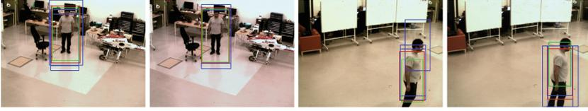
**Fig. 1.** Visualization of fusion system, the detector output is blue, tracker output green and the fused result red. The combination of both tracker and detector produces a more accurate bounding box estimate than the respective inputs, as seen in the first two frames. The last two demonstrate drift correction.
